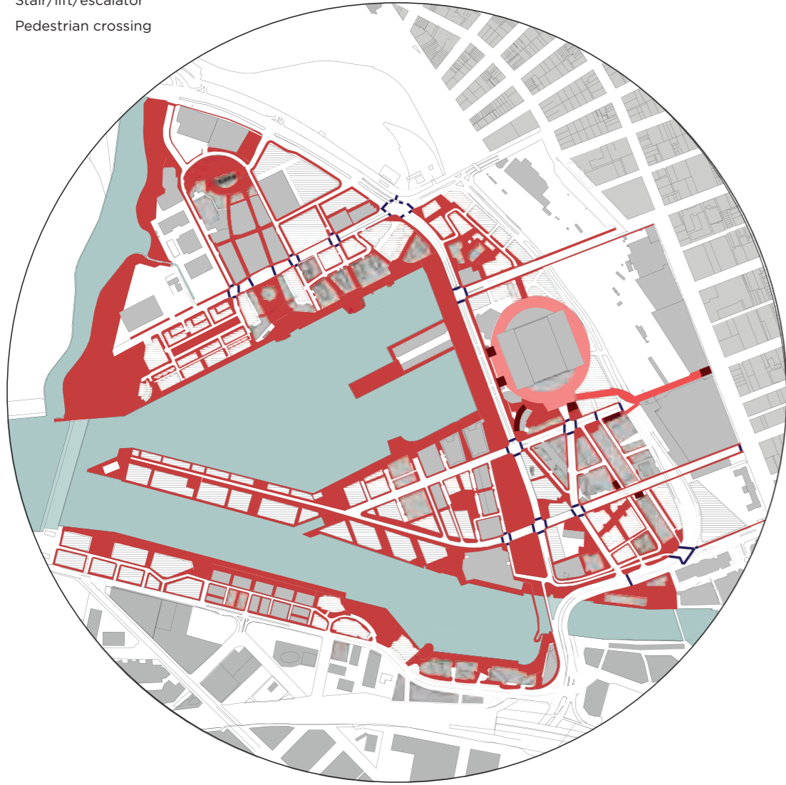
Fig 6.16 Existing and proposed pedestrian accessibility including level changes, stairs, lifts, escalators and key pedestrian crossings.
