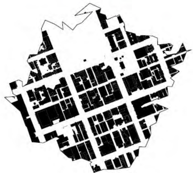
FIG. 35. Nollli Plan illustrating Net Catchment Area of built space (black) and unbuilt space (white).
