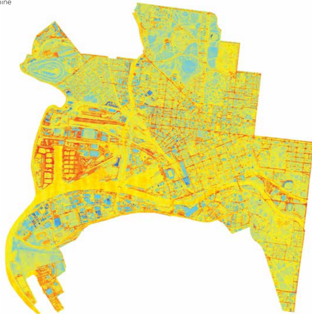
Thermal imaging of Melbourne, taken late at night, showing how paved, unshaded surfaces store heat from solar radiation and contribute to increased temperatures in urban areas.
