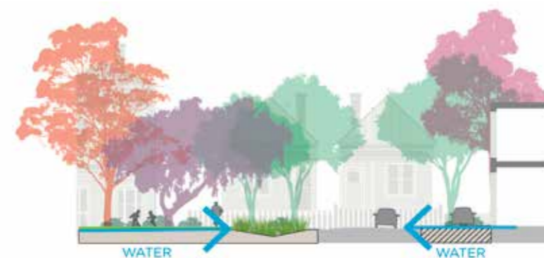
Water infiltration, permeable paving and structural soil or cells provide opportunities to grow larger, healthier trees in paved areas
