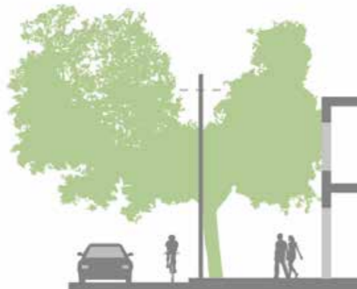
Tree trimmed under powerlines
