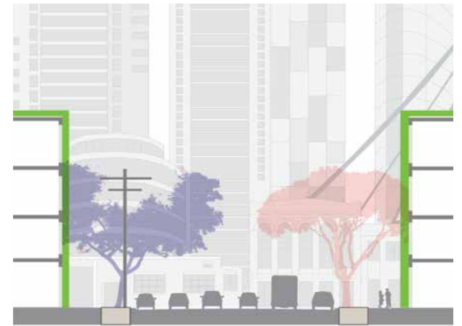
Trimming trees below low voltage powerlines
