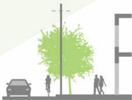
Small tree under powerlines
