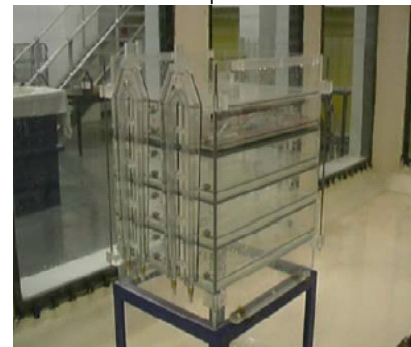
Figure 9. 1/35 scale model of a section of the CH2 building (Division of Fluid Mechanics, Department of Civil and Environmental Engineering, Imperial College, London)
