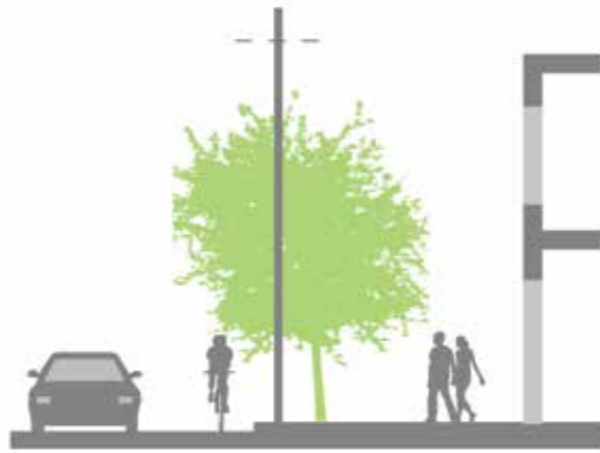
Small tree under powerlines
