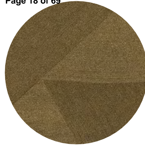
PF - BRONZE/GOLD COLOUR BRIDGE PAINT FINISH (AT ARCHES, BASE PANELS, VERTICAL DETAILS AS SHOWN ON ELEVATIONS)
