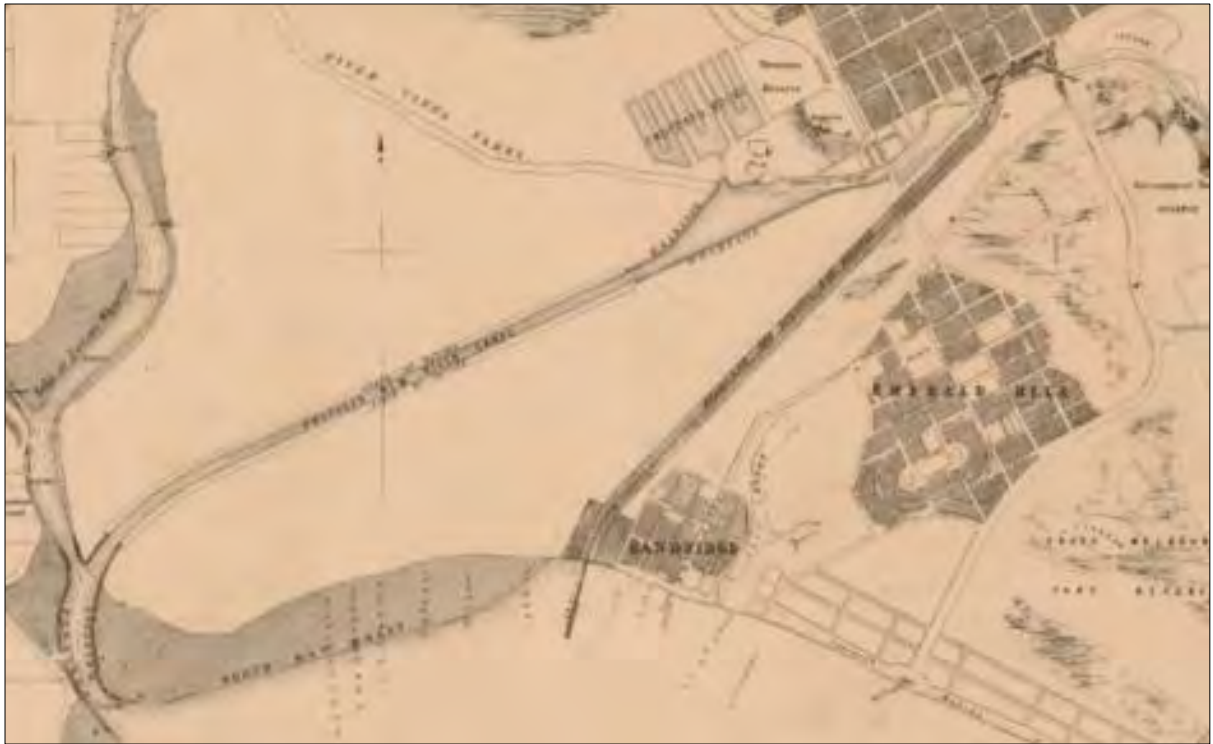
Figure 24—Plan of ship canal and site for docks, Robert Adams, Melbourne. Photo-lithographed by J.W. Osborne at the Department of Lands and Survey, 1860
