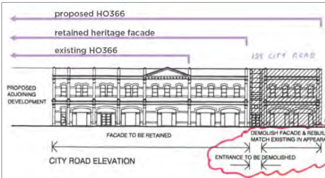
Figure 3 Extent of reconstructed building at 155 City Road and proposed extension of HO366
