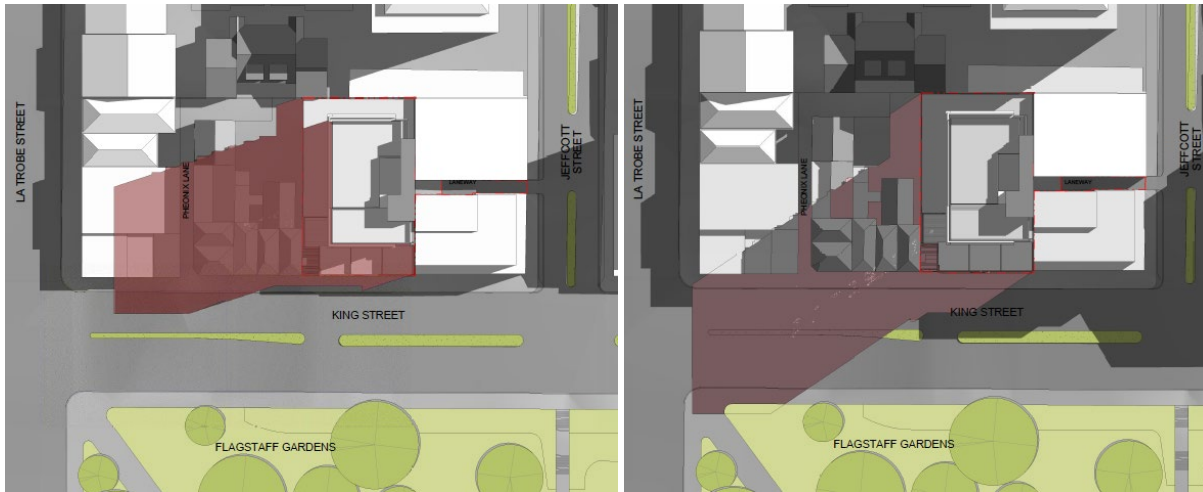
Figure 12 - 22 September Shadow Diagrams at 2pm (left) and 3pm (right). From Drawings S322 & S323
