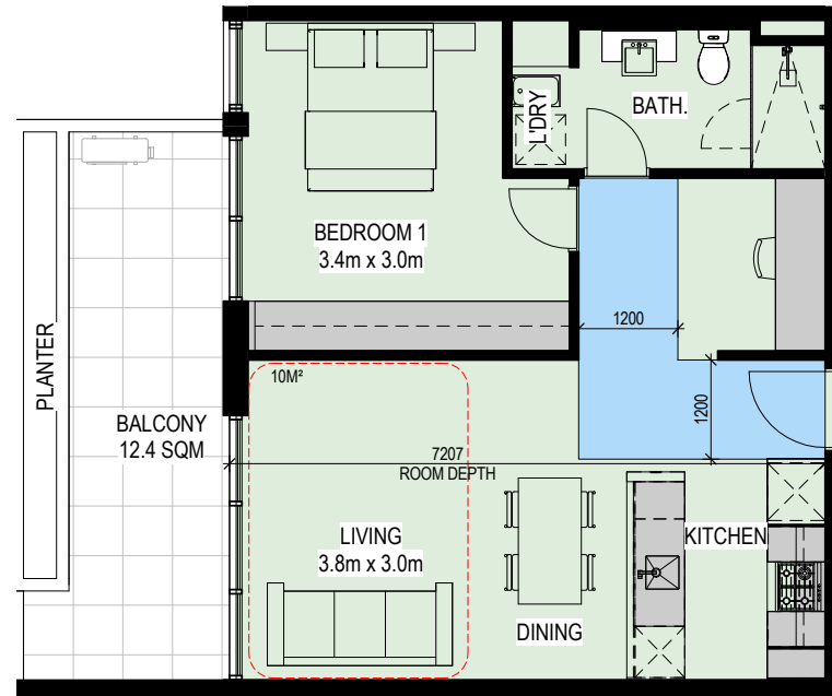
TYPE G 1 BEDROOM APARTMENT INTERNAL AREA - 50M 2 BALCONY - 12.4M 2 INTERNAL STORAGE - 7.3M 3 OVERALL STORAGE - 13.3M 3
