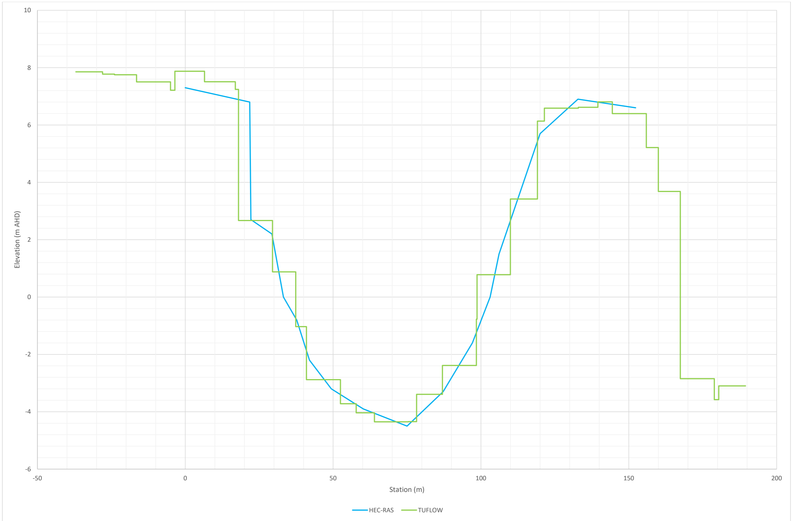
Figure 5 Cross-section immediately downstream of Morell Bridge (HEC-RAS Ch 11221, Spencer-Herr DS)
