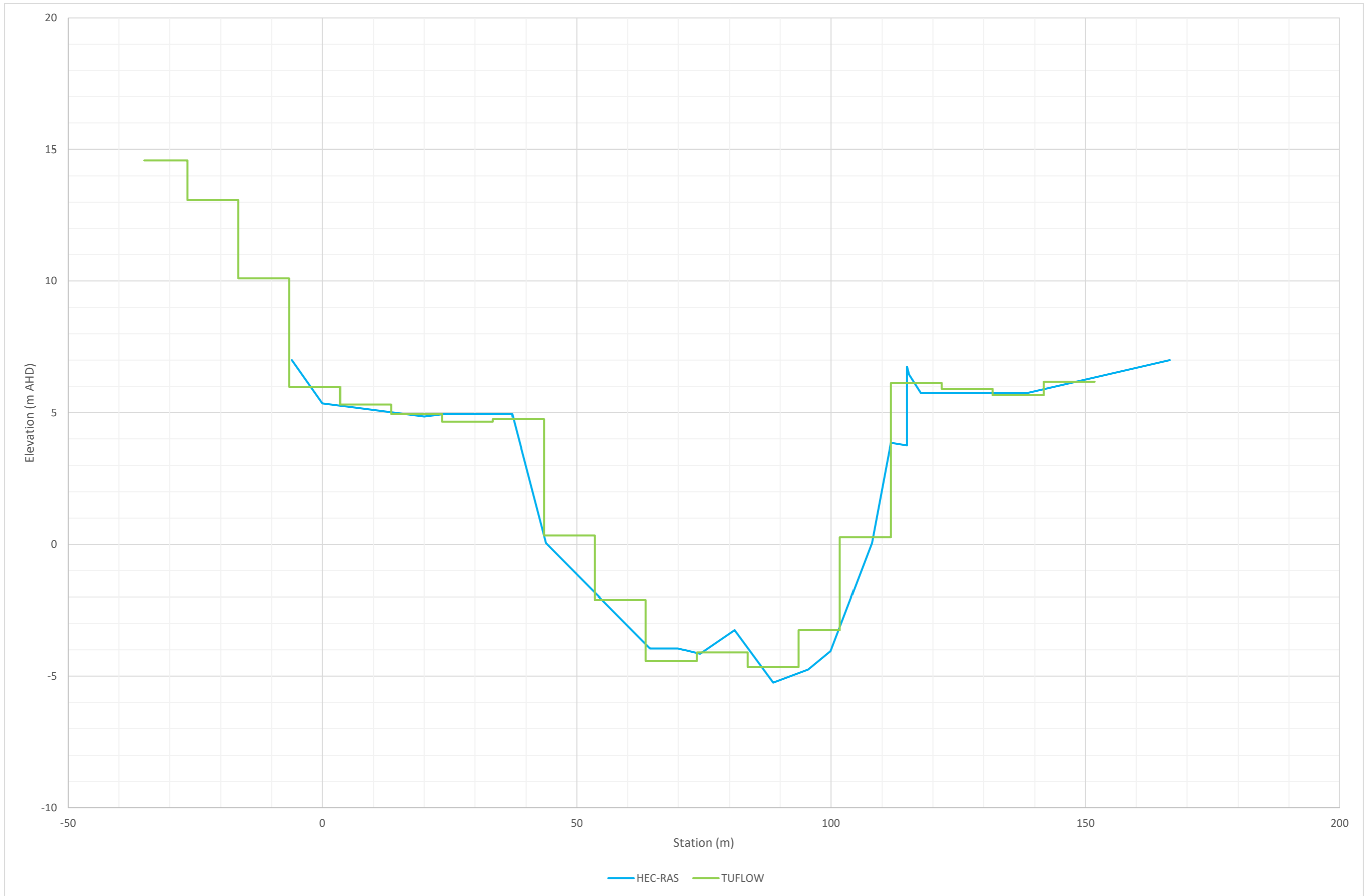
Figure 4 Cross-section comparison at between Herring Island and Church Street Bridge (HEC-RAS Ch 12877, Spencer-Herr DS)
