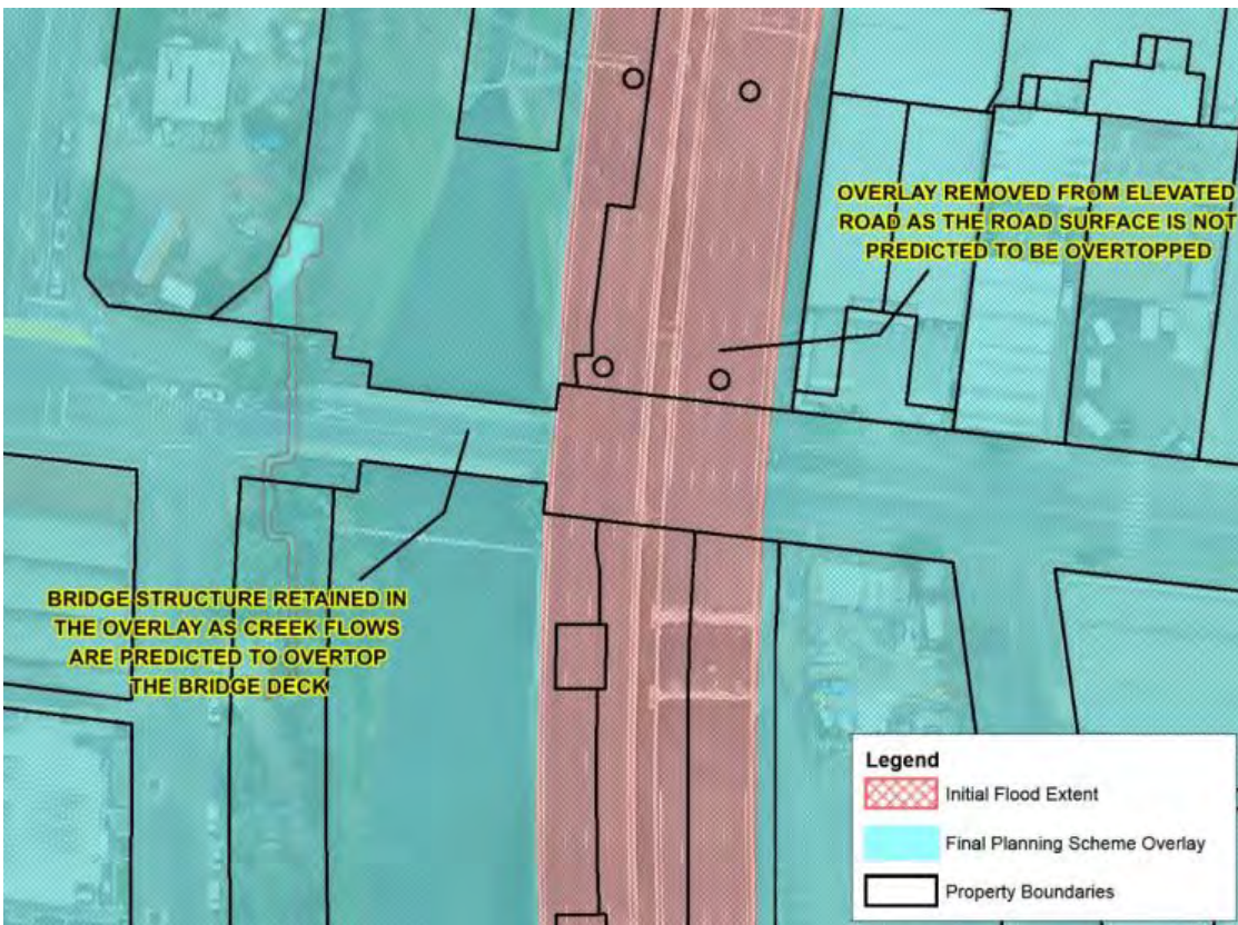
Figure 3.7: Example of bridge retained in the overlay, as well as elevated road removed from the overlay
