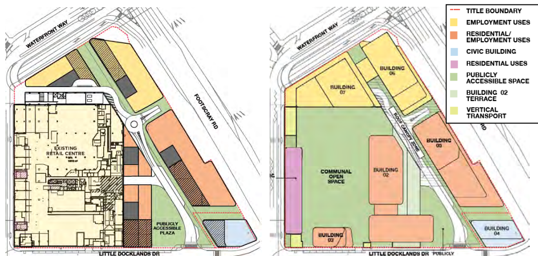
Figure 11 – Proposed DP Addendum extracts of ground and tower levels, depicting the proposed land use mix
