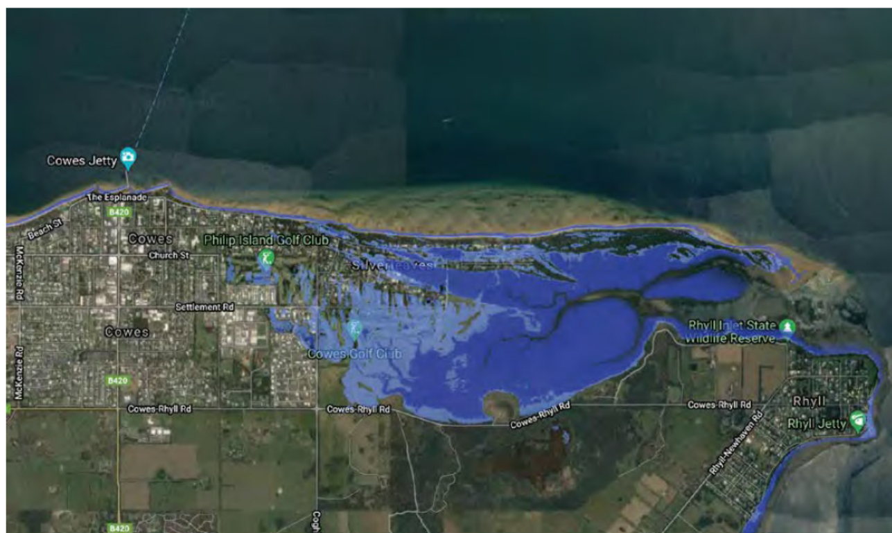
Figure 8: Predicted inundation risk modelling at highest tide for 2100 with +0.74m sea-level rise.
